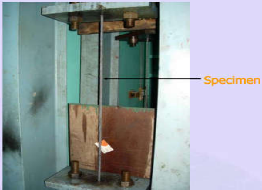
(b) Test of a seven-wire strand Set-up for relaxation test
