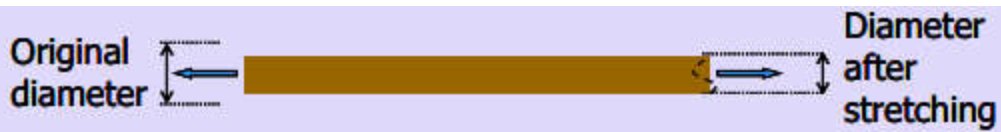
a) Applying tension to tendon
