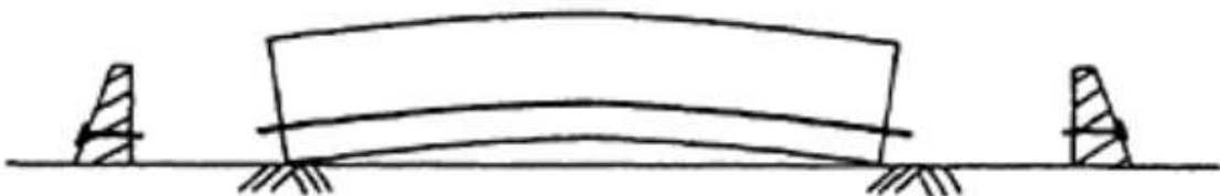
(c) Tendons released and prestress transferred
