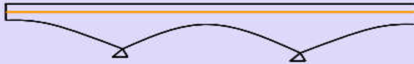
b) Varying level of soffit
