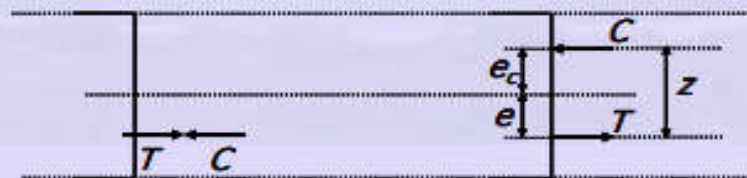
Internal forces at prestressing (neglecting self-weight)
