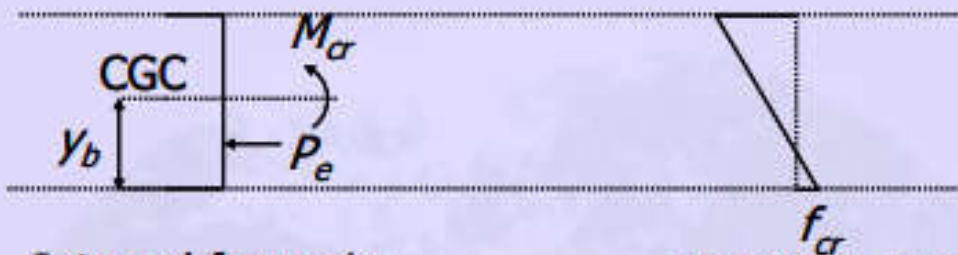
Internal forces in concrete
