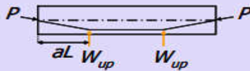
Free body diagram of concrete
