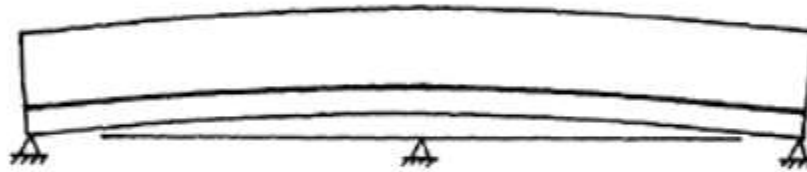
(b) Unrestrained deflection due to primary moment.
