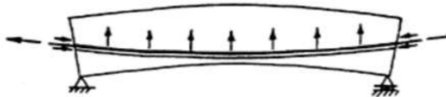
(b) Tendons stressed and prestress transferred
